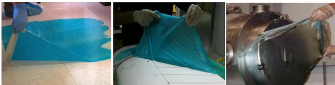
When dry, the product locks the contaminants into a polymer matrix. The film containing the encapsulated contamination can then be peeled. DeconGel peels from most non-porous and porous hard surfaces if the dried film is thick enough. If the film is difficult to peel, add another
