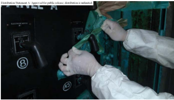
Figure 13. Dried DG can be easily peeled off from a variety of surfaces including bare concrete, three dimensional control panels and equipment, windows and walls.
