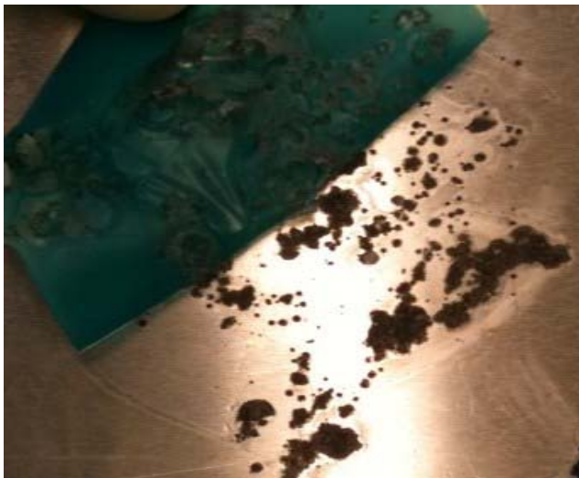
Figure 1. Aluminum powder reacted with the stainless steel surface creating a fixed Al surface deposit.
