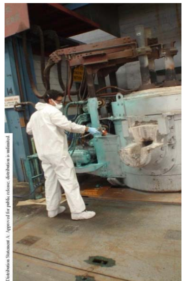
Figure 10. Sampling before decontamination and application of DG (1121) by spraying on vertical and three-dimensional surfaces.
