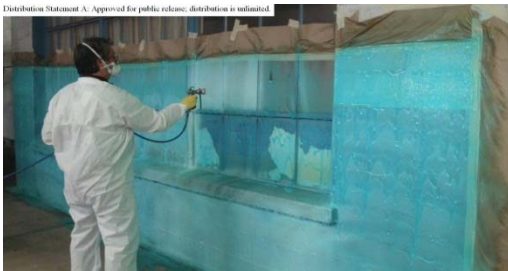
Figure 10. Sampling before decontamination and application of DG (1121) by spraying on vertical and three-dimensional surfaces.
