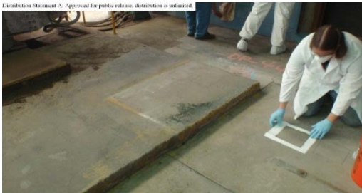
Figure 9. Overview of the large open floor area in Building 6 that DG was evaluated as a method of decontamination. The section consisted of a bare concrete area, a smelter with complex architecture, a control panel, painted concrete walls and glass windows.
