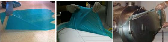
> Peel DeconGel off the surface by starting from one of the edges
