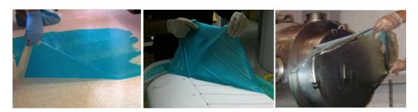
When dry, the product locks the contaminants into a polymer matrix. The film containing the encapsulated contamination can then be peeled. DeconGel peels from most non-porous and porous hard surfaces if the dried film is thick enough. If the film is difficult to peel, add another coat, let dry, and peel. In most cases the DeconGel will come off in a single sheet but for odd shaped surfaces you may be required to score DeconGel in order to peel it off.
